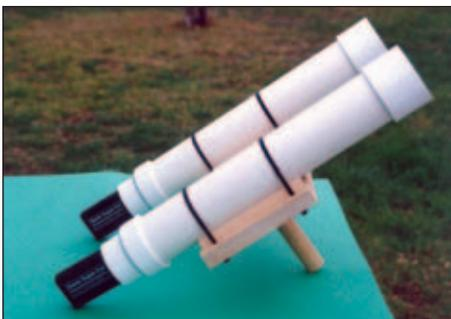
■ FIGURE 8. Pair of "Sonic Super Ears" used for the microphone/amplifier systems. The plastic case of one of the microphone/amplifier systems is shown cemented into a 2 x 1-1/2 inch PVC pipe increaser using Gorilla Glue.
